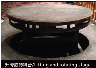
升降旋转舞台/Lifting and rotating stage
